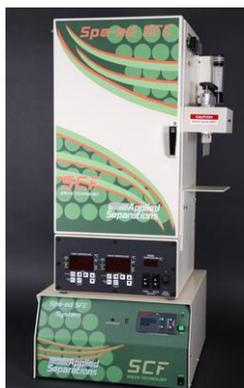
Supercritical carbon dioxide extraction of fats from chocolate products eliminates solvent cost, exposure to hazardous solvents, and additional solvent disposal costs.
